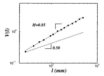
FIG. 5. Log-log plot of the normalized variance calculated along the y' for the high permeability zone of sample Lo, averaged over the three different faces of the sample. Along the y' direction, a correlation exponent of  $H\!=\!0.85\!\pm\!0.06$  is found. However, along the x' direction, a periodic pattern is observed. Thus the anisotropy in this sample is manifested in a change of behavior from long-range correlation scaling along y' to periodic morphology along x'.
