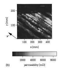
FIG. 2. (a) Photograph of the face z=0 of the sample Lo. The complete sample consists of two slabs of 448 mm by 246 mm and 10 mm thick, and again only three faces were used in this study. (b) Permeability map of (a). The permeability was measured every 12 mm and 4 mm in the x and y directions, respectively, so that a grid of  $n_x=38$  by  $n_y=61$  was obtained. Notice the strong anisotropy of this sample manifested by the crests elongated along the y' direction
